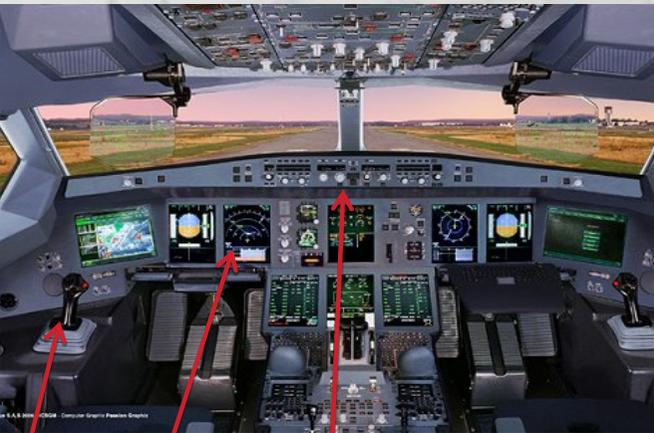
Sidestick LCD-Displays Autopilot, Auto-Throttle, Envelope Protection
